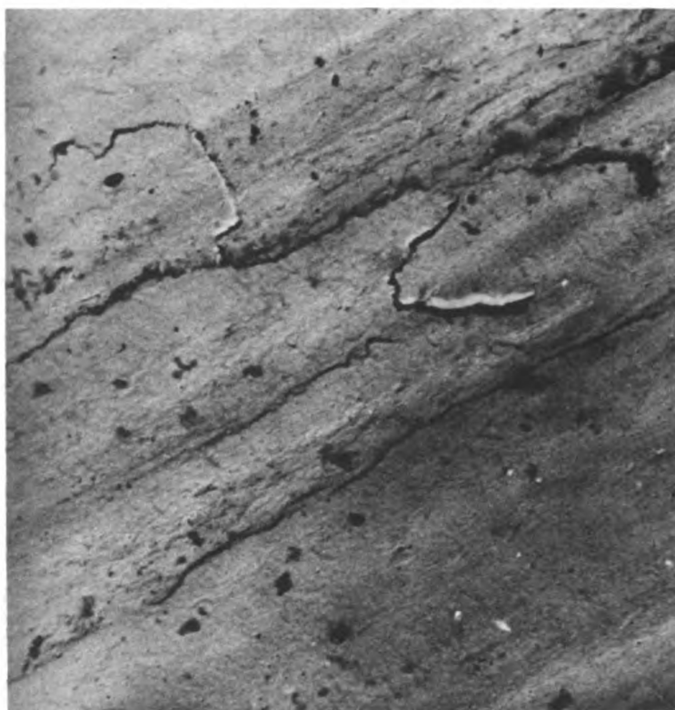
Figure 4b — Surface of wearing part. The smooth surface is composed of a sheer-mixed layer. Wear particles are in the process of breaking out.
