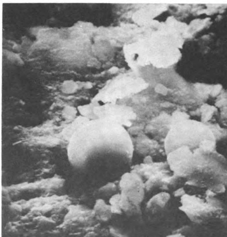
Figure 8a — Two spherical particles on a dense Ferrogram. The spheres are steel. The serrated particles behind the larger sphere are small laminar particles. Larger laminar particles such as the one shown in Fig. 8c are easier to distinguish from rubbing wear particles. The combination of spheres and laminar particles occurs when fatigue causes micro cracks in a race or ball.
