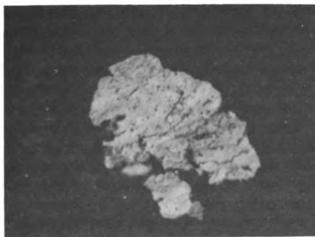
Figure 8c — A lamellar particle. Such particles are often twenty or more micrometers across. Lamellar particles are generated when a ball rolls over a metal piece. The resulting particles often has holes in its surface and serrated edges as the result of stretching the metal.
