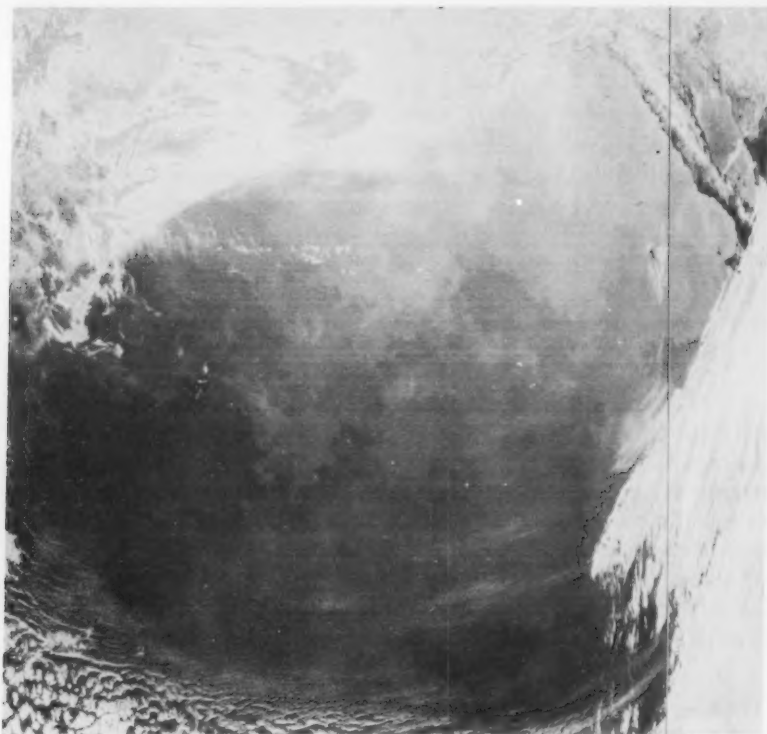
Figure 6 — NOAA satellite Very High Resolution Radiometer, infrared image, 14 December 1974. Central Pacific region. A large outbreak of continental air moved west from Southern California/Baja California (to the far east in the image) to provide good imaging condition for detection of mesoscale temperature gradients featured on the sea surface, the subtropical convergence of the North Pacific.
