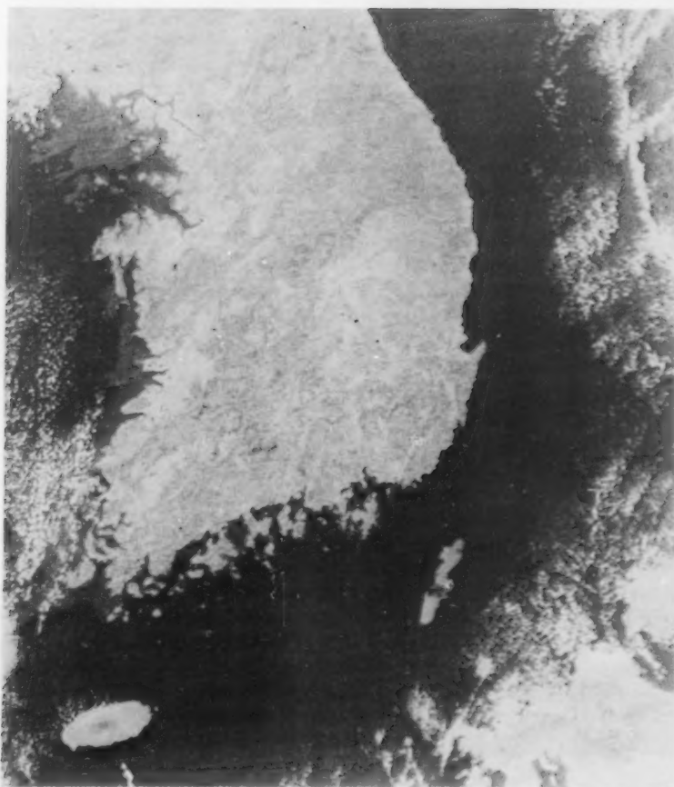
Figure 1 — Direct readout visual and infrared imagery from the Defense Meteorological Satellites. a) VHR visual (0.6 km spatial resolution) image, a small portion of the full swath showing the Korean Peninsula and surrounding oceanic areas.
