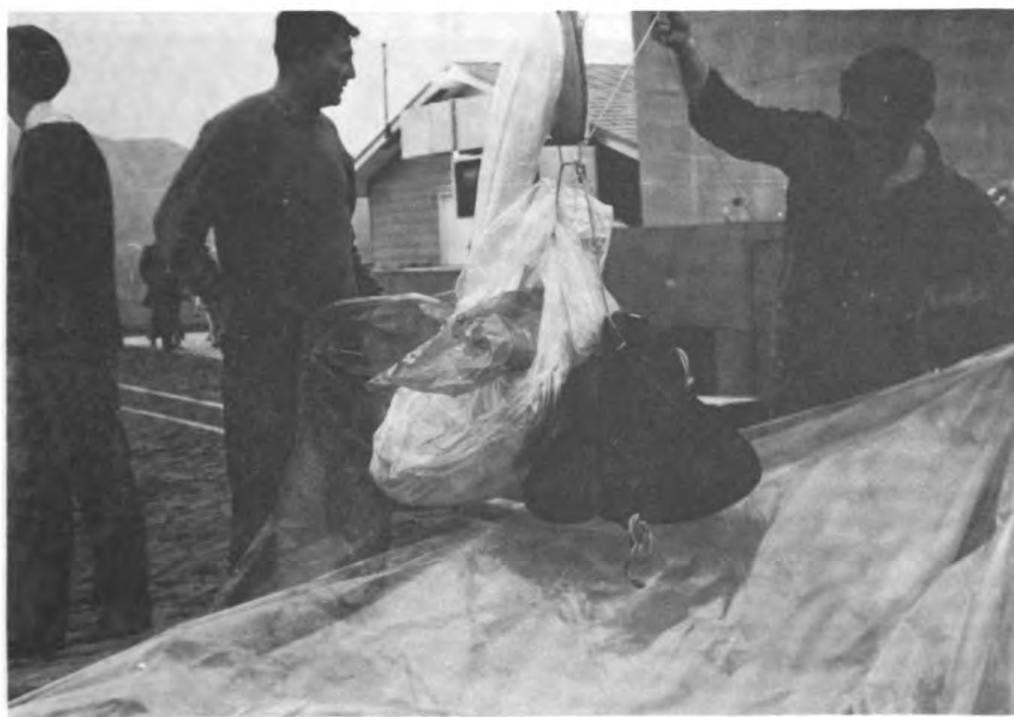
Figure 6 — Weighing off using the Huch Clutch technique. The inflation proceeds until the entire system weight, including free lift for ascent is just neutrally buoyant. The dark sleeve at upper center is the clutch, which is removed prior to launch by hand.
