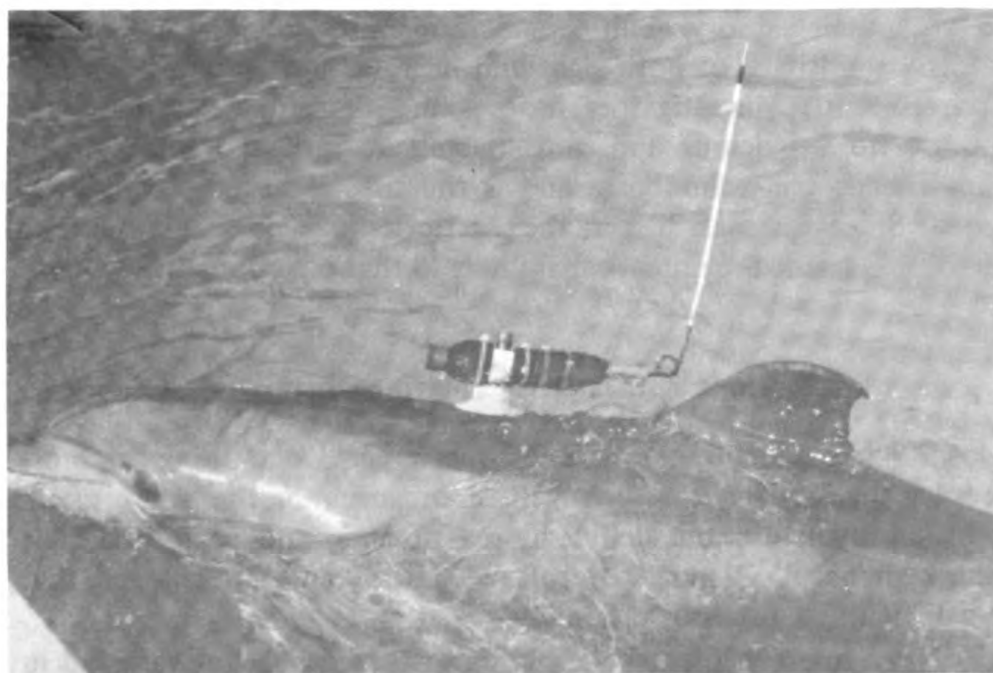
Figure 7 – Attachable radio transmitters for smaller whales. (a) Early model was attached to dorsal fin of porpoise; hydrodynamic problems are obvious. (b) Newer model is attached with suction cup and mounted on a swivel; rides in precisely the position occupied by a baby porpoise accompanying its parent. (Photos courtesy Dr. William Evans, Hubbs-Sea World Research Institute, San Diego)
