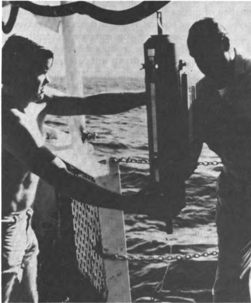
Figure 1 – The traditional method of sampling by bottle limits the resolution with which chemical variables can be measured in the ocean.
