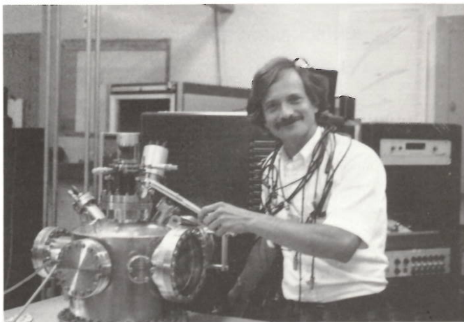
Dr. Singer, one of the authors, is shown wrapped up in a Scanning Auger microprobe used to study the composition of implanted bearing steels. With Auger analysis and ion-milling, the relative abundance of most elements above helium can be determined to a depth of several thousand Angstroms.
