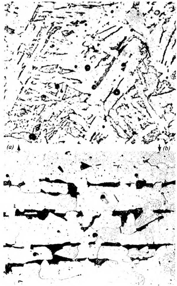
Figure 14. Microstructure of Mild Steel Laser Beam Weldment (a) base plate and (b) fusion zone.
