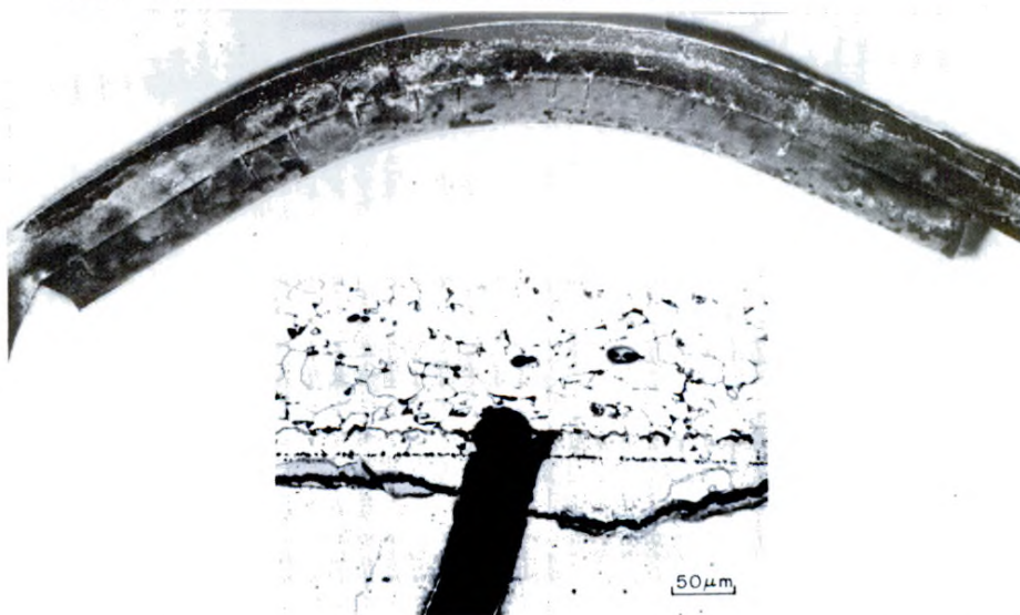
Figure 15. A 1.3% UHC steel/mild steel composite after "selective-heat-treatment" (770°C for 20 minutes then water quenched) is bent until cracks in the martensite portion of the composite become visible. The photo-micrograph shown above illustrates that the crack in the martensite region is arrested in the mild steel region. No delamination is noted in the interface region indicating that a good metallurgical bond is present in the laminated composite.
