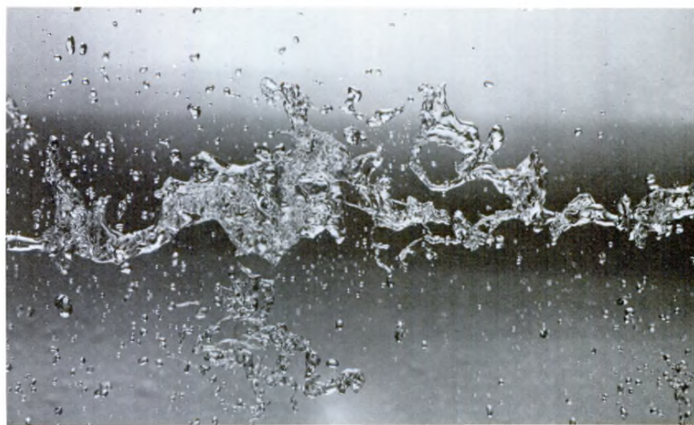
Figure 11. All cohesiveness is lost as the jet breaks up. (288 diameters downstream.)
