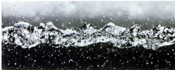
Figure 6. Water jet surrounded by spray. Helical motion can be detected. (144 nozzle diameters downstream.)
