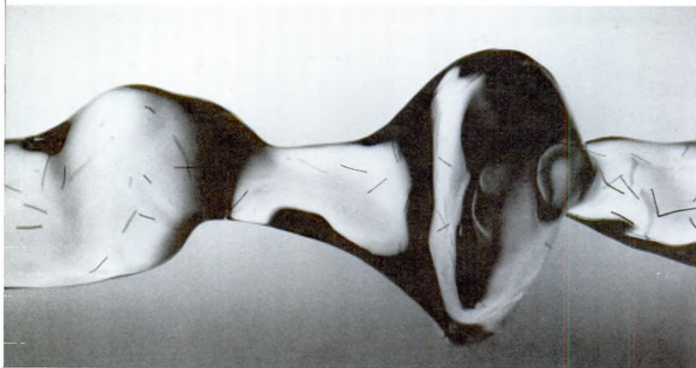
Figure 13. The helical phase in a jet designed to avoid axial instabilities.
