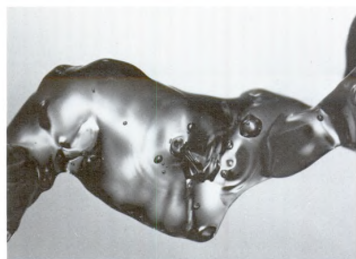
Figure 8. Air bubbles breaking out of the jet surface leave circular ripples.
