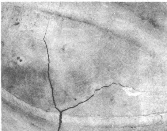
Figure 4. Close-up of weld fracture caused by explosion.
