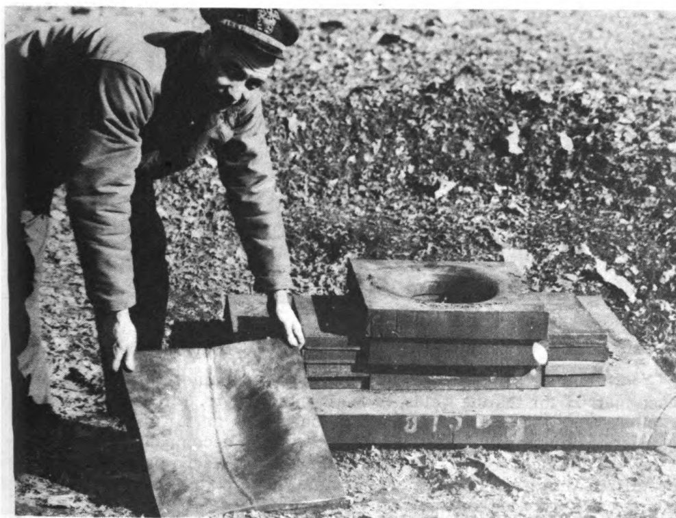
Figure 1. Result of a welding test by new method.
