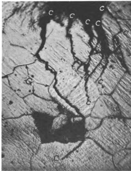
Figure 3. This photomicrograph of low-carbon steel shows fatigue cracks beginning at small corrosion pit. The fine cracks designated by "C" propagate across the grains on certain preferred planes which differ in orientation for the various crystals. G indicates a grain boundary of a crystal.
