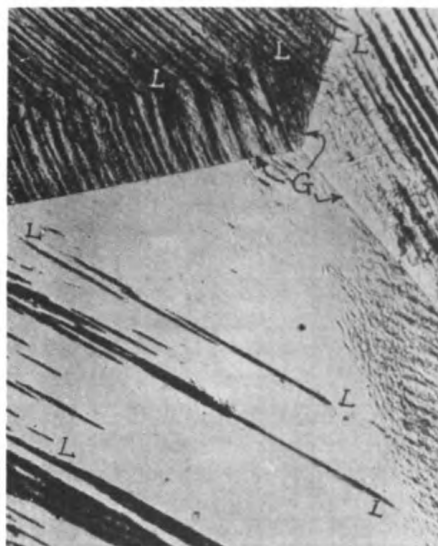
Figure 7. Photomicrograph of slip bands in crystals of high-purity aluminum after repeated stressing. (G is a grain boundary, while lines designated "L" are slip bands.)
