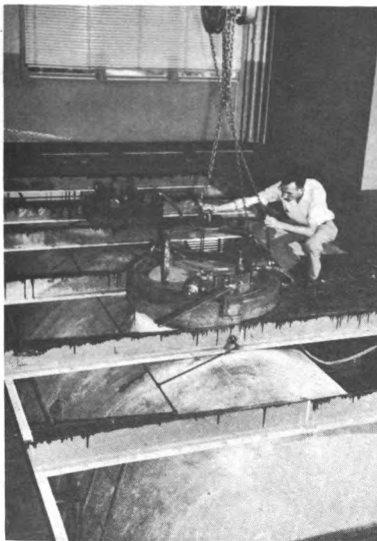
Figure 2. This high-pressure tank is used for testing the ability of submarine sonar equipment to withstand the pressures of deep submergence. The tank is built of four-inch-thick steel to withstand pressures of 1000 pounds per square inch, corresponding to a sea depth of 2000 feet.
