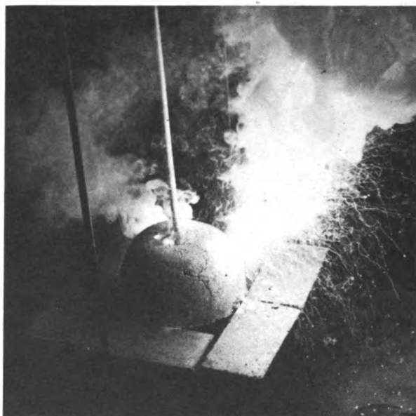
Figure 1. Spherical furnace for burning metals in oxygen
