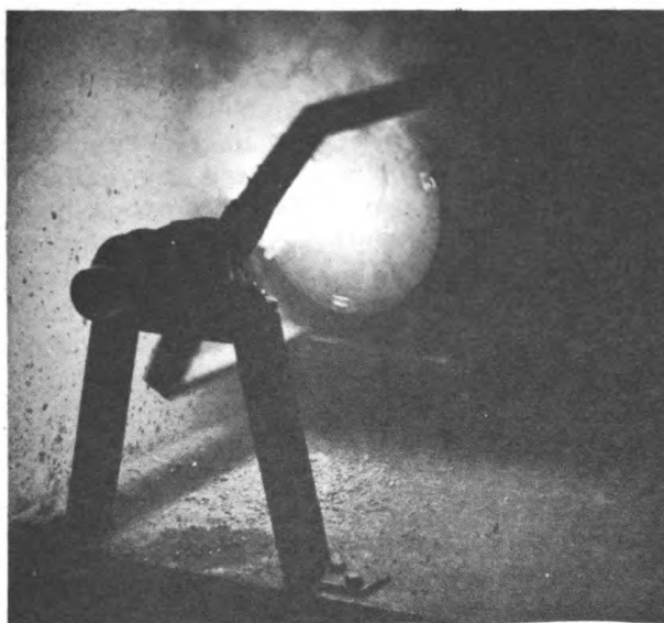
Figure 3. Centrifugal reactor in action-- burning aluminum in oxygen
