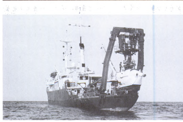
Mother ship Atlantis II recovers Alvin after a dive. Atlantis II is Alvin's second and current mother ship.
