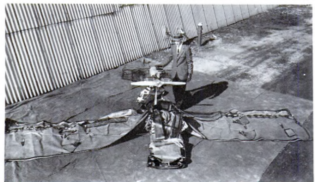
The spread out inflatoplane ready for inflation
