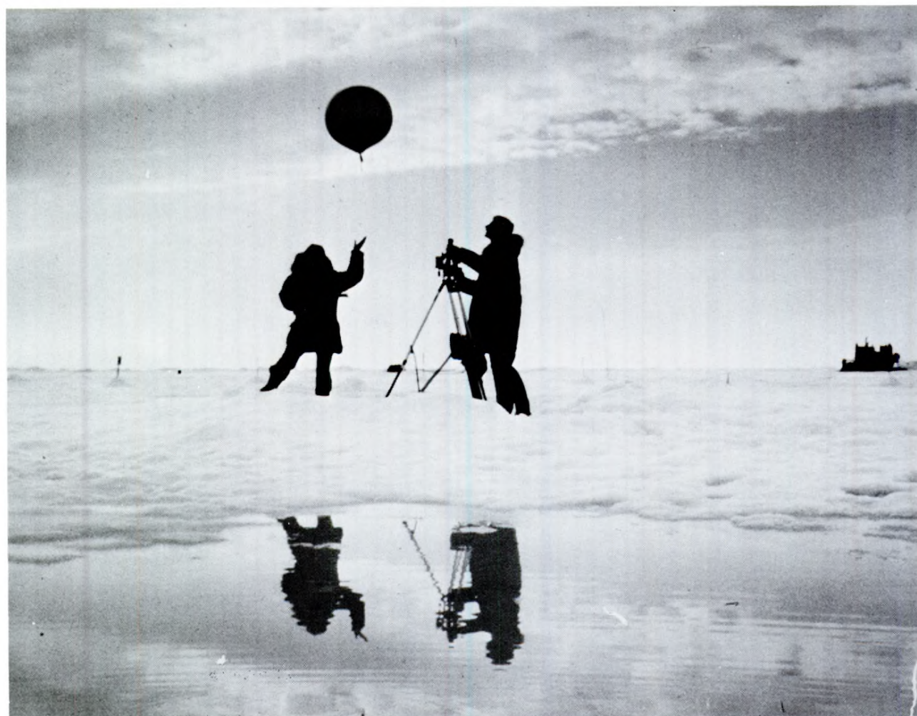
A meteorologist releases a balloon for wind profile measurement while another tracks it with a surveying instrument in the 1970's. Future tracking will be done by the Global Positioning System (GPS).
