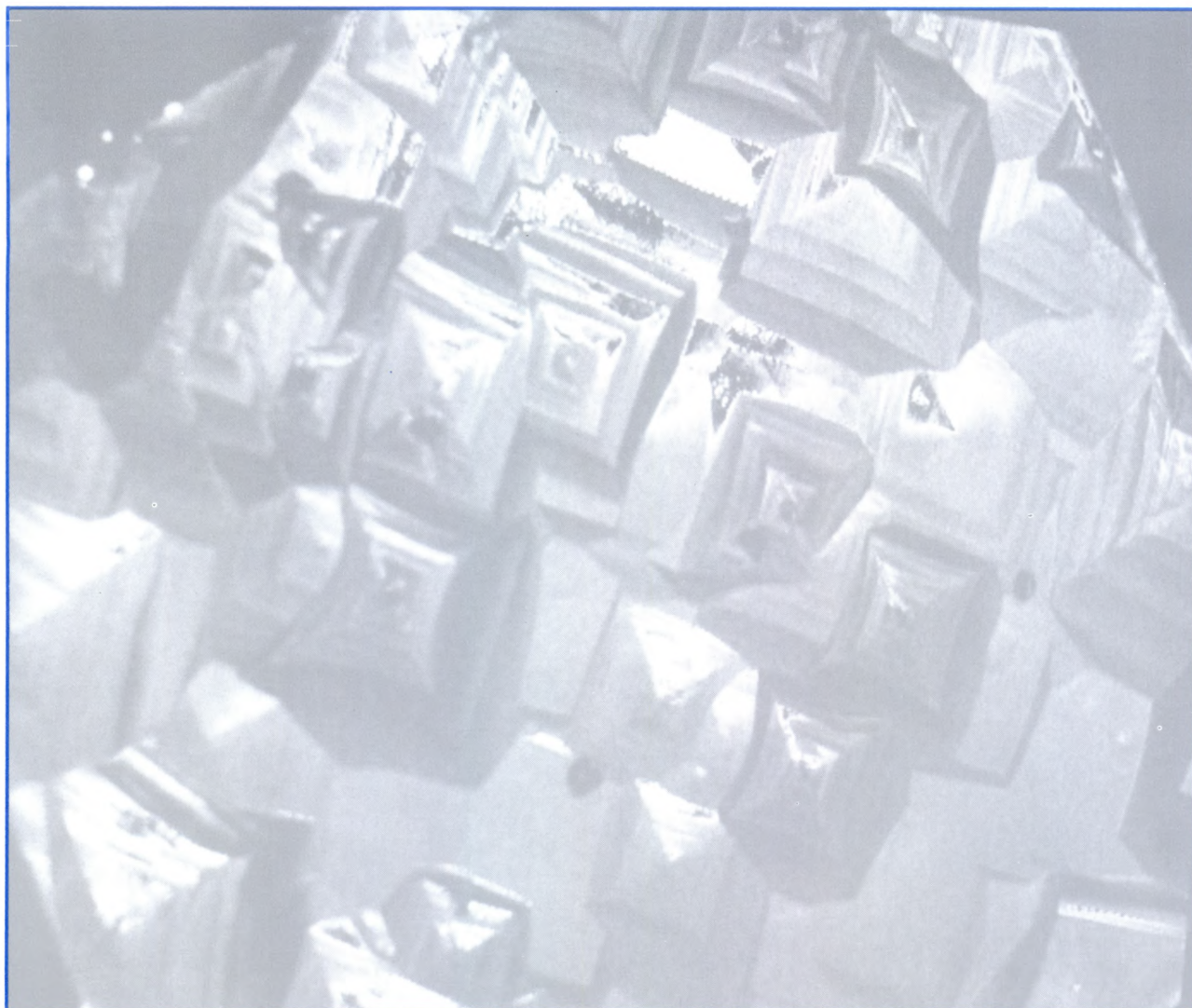
Scanning laser microscope image of homo-epitaxial diamond grown on a diamond seed crystal using an oxygen-acetylene torch in atmosphere. This research is part of an ongoing study funded by the Office of Naval Research to better understand how diamonds grow. Single crystal diamond films may form the basis of high speed, high temperature, radiation hard micro-electronics.
