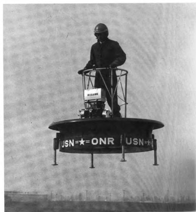
The "Flyer Platform" built by Hiller Helicopters for ONR in 1955 levels off in free flight. It is the first aircraft using a ducted fan for lift and propulsion to attain free flight.
