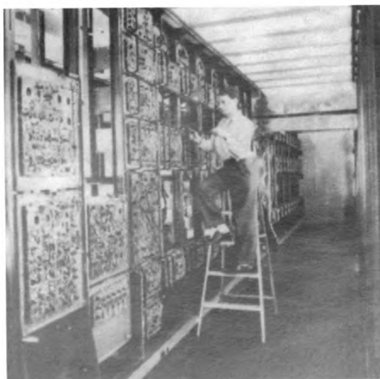
ONR sponsored the development of the first full-scale digital computer to utilize magnetic core memory. The project known as "Whirlwind" began in 1946 resulted in a computer which remembered, acted upon, and delivered information at a rate of 20,000 times a second; a record achievement for the day. The "Whirlwind" computer filled a room when it was completed.
