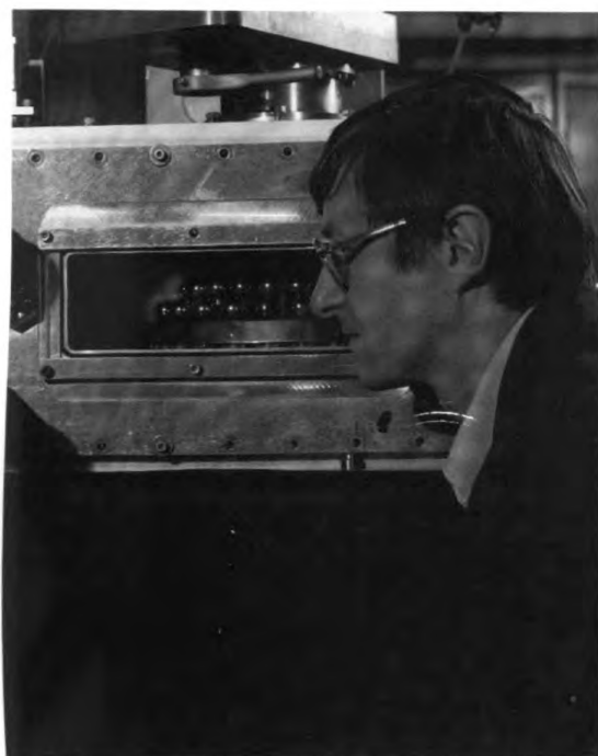
Dr. Graham Hubler of Naval Research Laboratory examines the rolling elements of a J-79 bearing during ion implantation with chromium ions. The glow is caused by fluorescence of highly excited atoms sputtered from the surface of the 150-keV chromium ion beam. Ion implantation consists of injecting atoms of any desired element electronically into the surface layer of a metal, producing an intimate alloy without the sharp interface characteristics of a coating. This technique can make wear-resistant parts that increase manyfold the lifetime of the engines or systems in which they are used.
