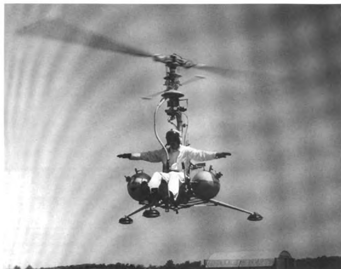
The Kellett KH-15, dubbed "Stable Mable," which was rocket-powered, flew in 1953. Stable Mable incorporated gyrostabilizing controls designed to give helicopters greater stability in the air and cut vibration.
