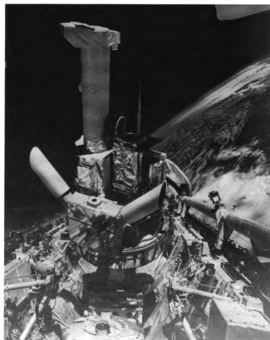
Two Naval Research Laboratory solar experiments were flown on the Space Shuttle's Spacelab 2 in 1985. Shown here is the high resolution telescope and spectrograph (HRTS) which was designed and built by the Naval Research Laboratory to measure the ultraviolet radiation from the sun. NRL astrophysicist Dr. John David Bartoe was aboard Spacelab 2 as a payload specialist.
