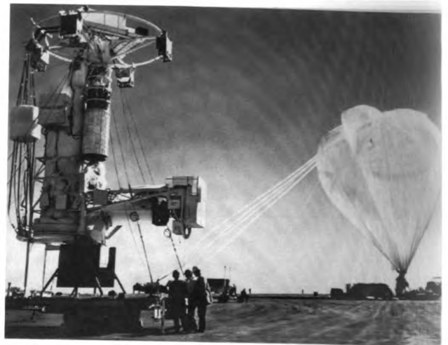
The Stratoscope II telescope, which was funded by ONR, is shown in launch position in 1963 during inflation of its carrier balloon. The launch balloon is filled with 350,000 cubic feet of helium. The telescope, lofted to an altitude of 80,000 feet, operated above 98 percent of the air and water "blanket" that surrounds the earth, and data was obtained free of the absorptive effects of the atmosphere. The balloon-borne telescope collected new and vital data on Jupiter and the giant, red stars
