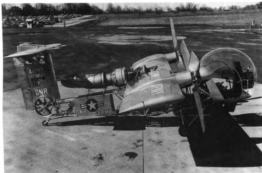
This unique tilt-wing aircraft was built by Vertol Aircraft Corporation for the Army under the direction of ONR. This Vertical Take Off and Landing (VTOL) aircraft was designed to take off and land vertically, hover, and fly forward without any ground run. This aircraft is a research milestone in the development of the V-22 "Osprey" tilt-rotor plane of today.
