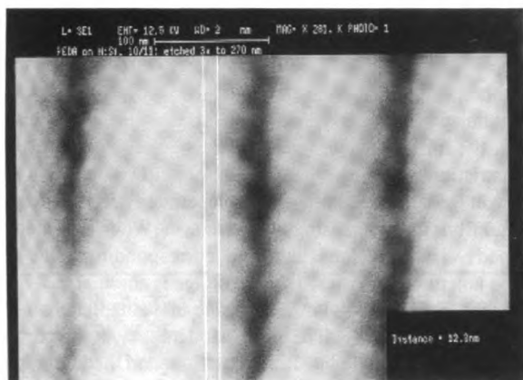
Figure 7 Narrow trenches etched into Si created by the process illustrated in Fig. 6.
