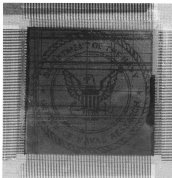
Figure 2 A reflective Ch-LCD made from plastic substrates with polypyrrole electrodes.
