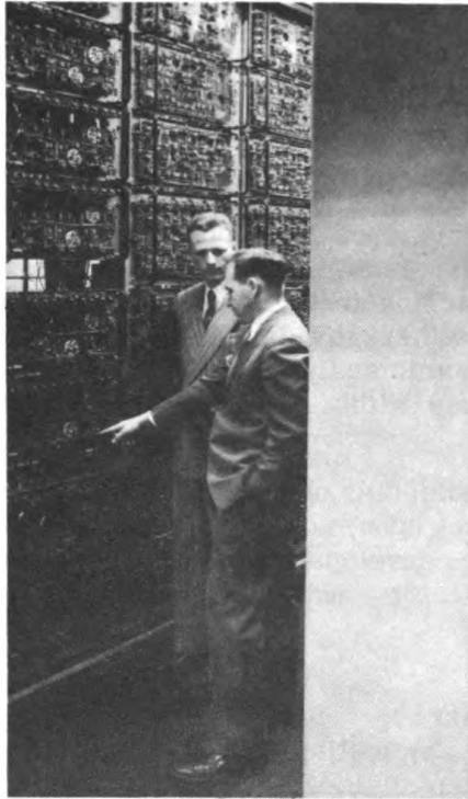
Figure 2. The arithmetic element of Whirlwind I is examined by Jay W. Forrester and Norman H. Taylor, who heads Electronic Development.
