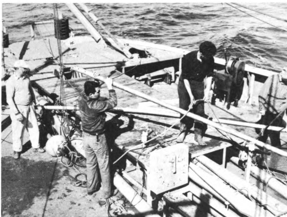
Two sections of bottom corer being rigged on the Horizon (a Scripps Institution Ship). The top section of the corer rests on the deck near the feet of the author, left.
