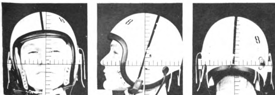
Figure 4. Comparison photographs of helmet No. 7, which were taken to show the amount of protection the headgear afforded.
