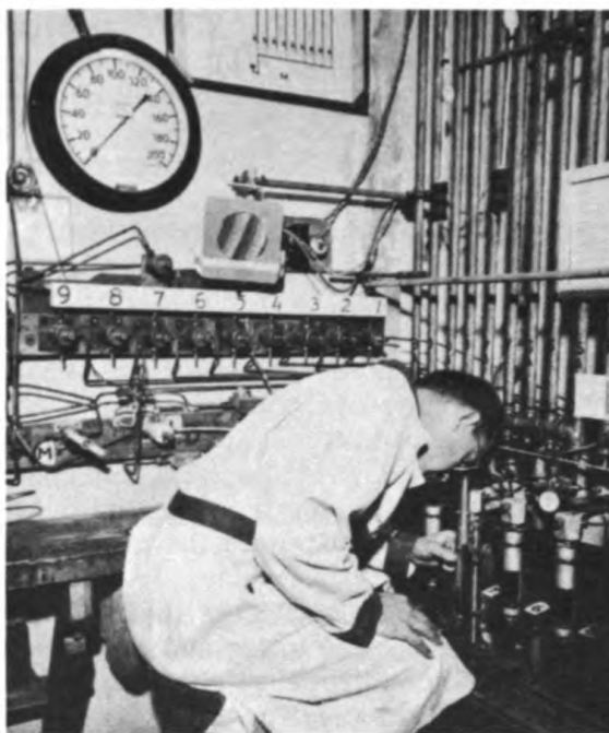
Lower end of the multiple tube manometer in operation at University of Wisconsin.
