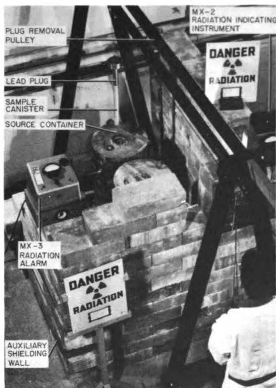
This technician is remotely lowering a plug and sample canister into a lead "pig" containing a 1,000-curie cobalt radiation source. Note reading on radiation instrument at right.
