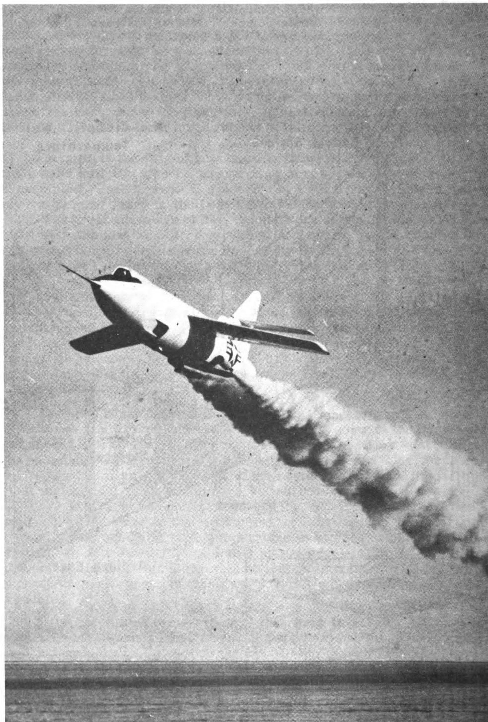
Figure 5. Here the supersonic Douglas Skyrocket (see cover) takes off under its own power. It can do this only when a jet engine has been installed; normally it is powered by rockets. Its top speed is secret. The type of take-off shown here has the disadvantage of sharply limiting the range of the Skyrocket.
