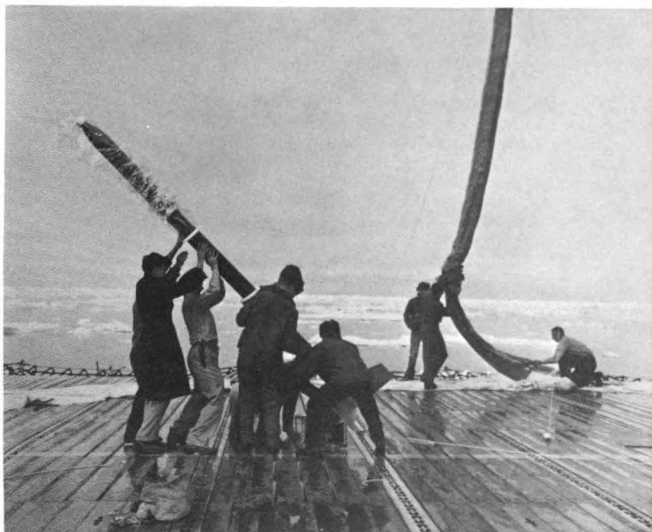
At right, the sleeve is being removed from the partially inflated balloon. At left, the rocket is being raised and covered with a plastic "Green-house" to keep it warm. Below the rocket is the automatic timing device.
