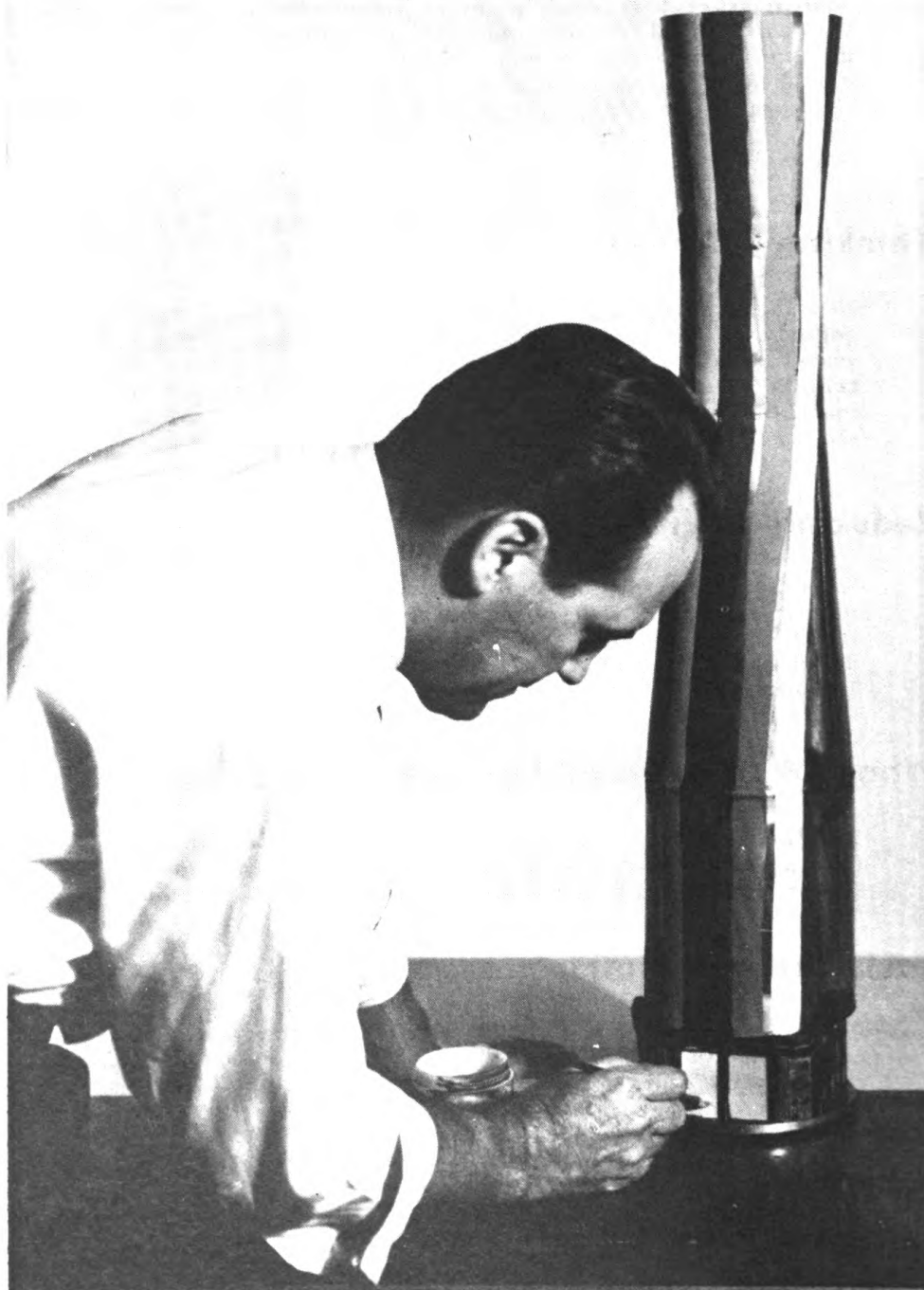
Temperature-indicating paint is being applied to a pulsejet engine prior to operation. By the changing color of the paints, the outside temperatures of the engine are revealed.
