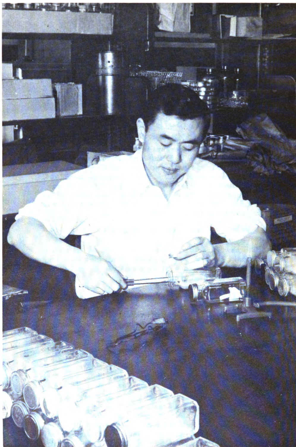
Determination of decay resistance is one of the screening tests applied to tropical woods. The graduate student-technician above is placing specimens of wood under exposure over pure cultures of brown-rot and white-rot fungi.
