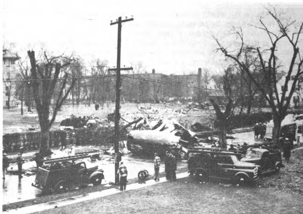
Crash of National Airlines DC 6 at Elizabeth, N. J. In the center background is the top of the building struck by the plane. The wreckage of the wings, engines, and forward half of the cabin is strewn in the open field. In the foreground is the rear half of the cabin, broken in two by its impact with a large tree. Thirty-two passengers survived, 27 were killed. All but four of the strong belts held, and there was no evidence of injuries attributable to belts.
