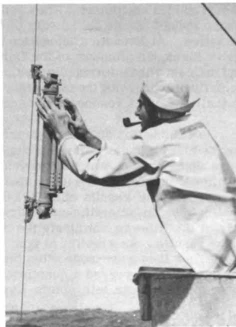
Preparing to lower a sampling bottle to obtain data on temperature and salinity at great depths. (Photograph, courtesy of Scripps Institution of Oceanography)
