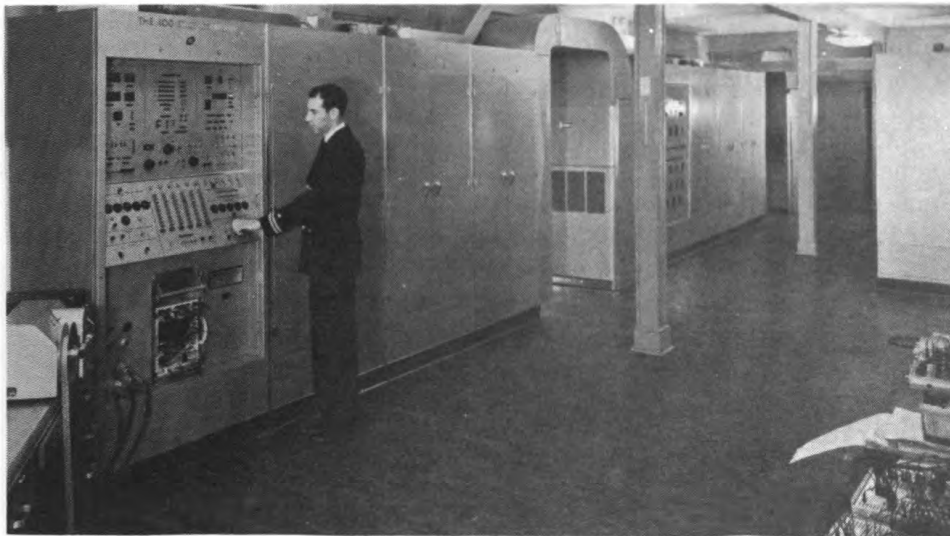
LT Robert J. Rossheim, USNR, is adjusting a knob on the operating panel of the computer. The tape reader (on the desk at lower left) feeds data into the computer by means of punched paper tape. Plug boards, the nerve centers of the computer (shown at the lower right) are wired in advance for a particular problem, then placed in the lower central area of the operating panel.
