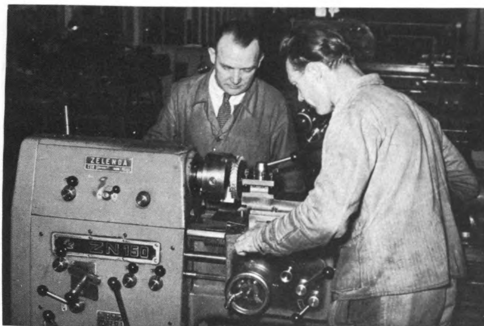
Here a metal wheel is being machined. This operation takes place after presintering, when the hard metal has a consistency similar to that of graphite.
