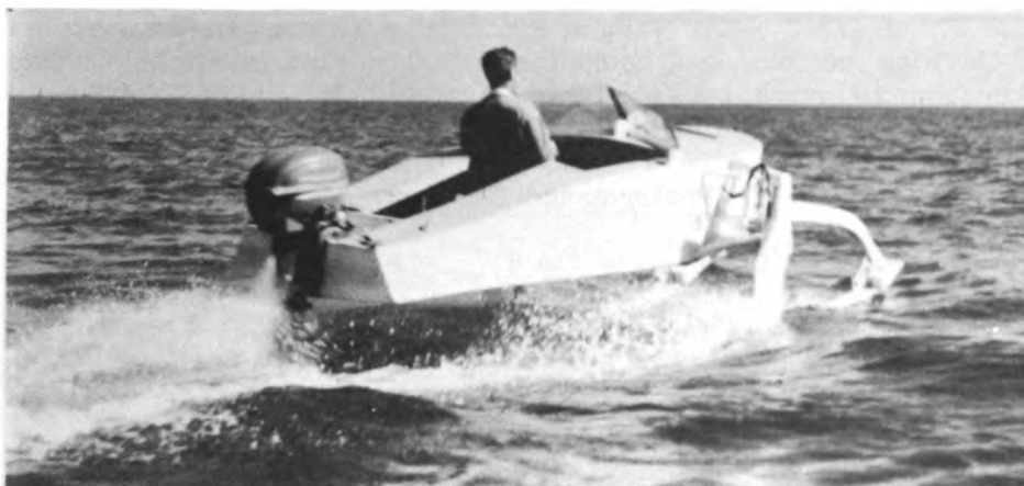
The Hook "Hydrofin" powered by an outboard motor makes a speed of about 25 mph.
