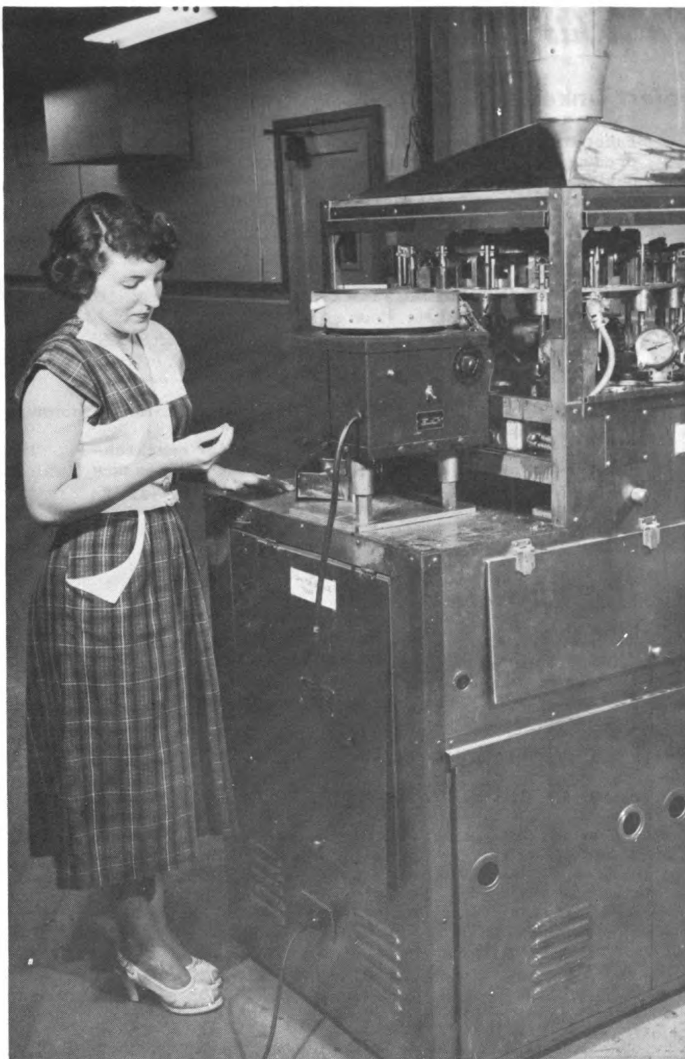
The young lady above is examining a titanate capacitor made by the Bureau of Standards mechanized system of producing electronic parts. The capacitor has just gone through the machine, which automatically deposits a thin coating of solder on silvered portions.
