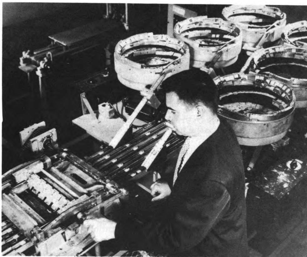
Robert L. Henry, Bureau of Standards project leader, and the wafer pattern printer. Mr. Henry is pointing out the special mounting for a stencil screen bearing circuit patterns.
