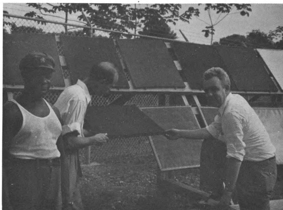
Figure 5 - Weather-coated fabrics on exposure to direct sunlight at the Tropical Exposure Site
