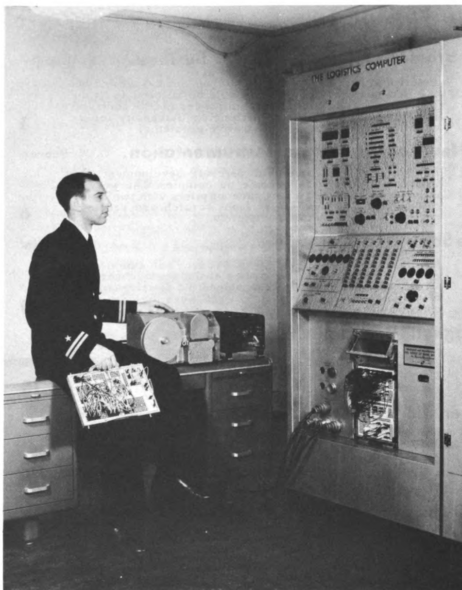
Control panel and some input equipment of the Logistics Computer - George Washington University
