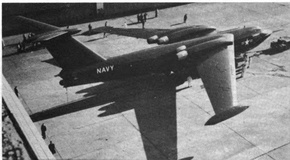
Figure 3 - Reinforced plastic wing-tip floats of the "Seamaster," a Navy seaplane (XP6M) do not corrode and require only simple maintenance (Photo courtesy of The Glenn L. Martin Co., Baltimore, Md.)
