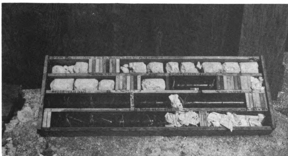
Figure 3 - Light-colored limestone cores (above) and dark basalt cores (below) obtained from depths of more than 4000 feet under Parry Island.
