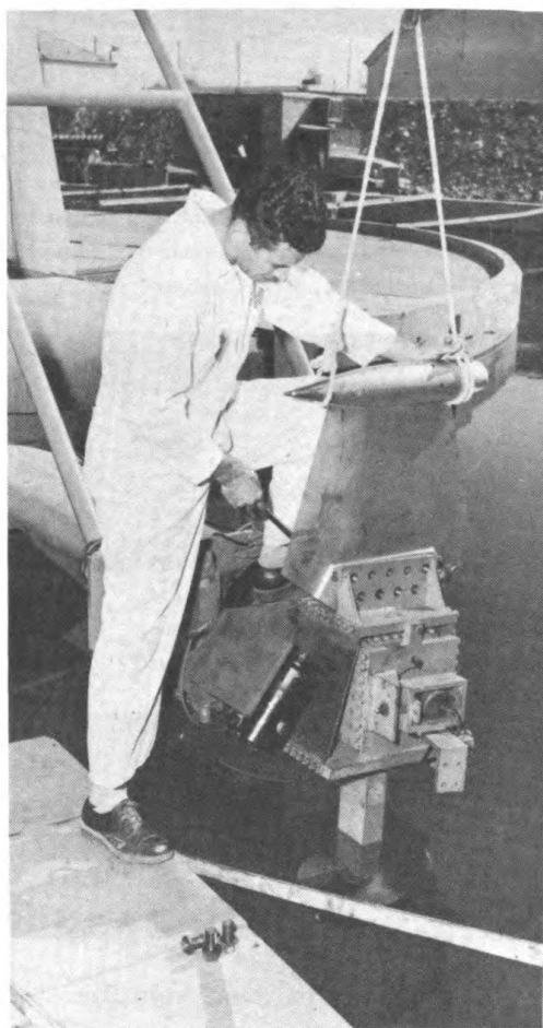
Installation of model on mechanism which allows attack angle to be varied during test.
