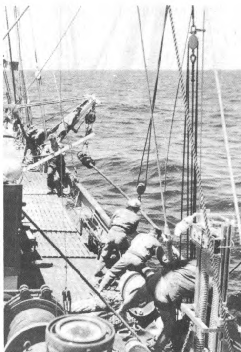
Figure 3 - Coring rig being prepared for lowering.
