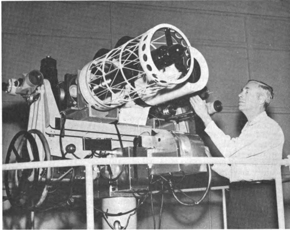
Figure 5 - Askania theodolite cameras collect optical data during missile flights. Camera at left has no lenses, but uses mirrors, like a telescope, to reflect light and put an enlarged image on film.
