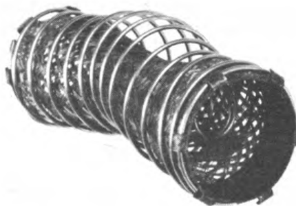
Figure 4 - "Chinese handcuff" shield for Model I Series packages. Formed of soft copper braid blackened for good heat transfer, the shield is held in intimate contact with tube walls by spring action.
