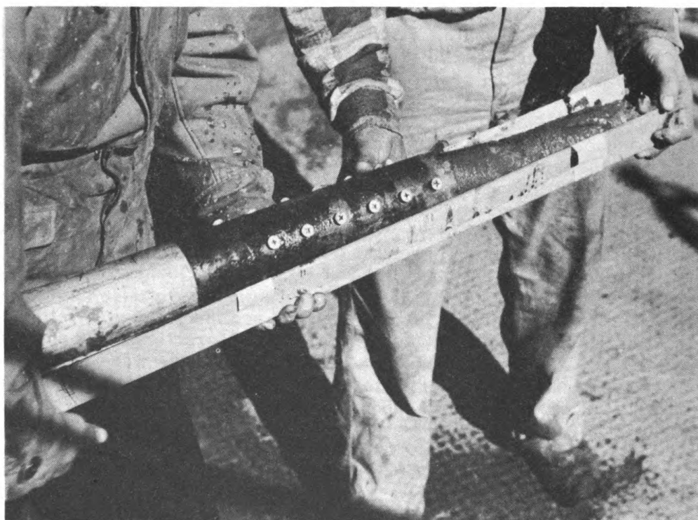
Figure 2 - A core of sediment lifted from the floor of the ocean is being slipped out of the Kullenberg piston-type coring device.
