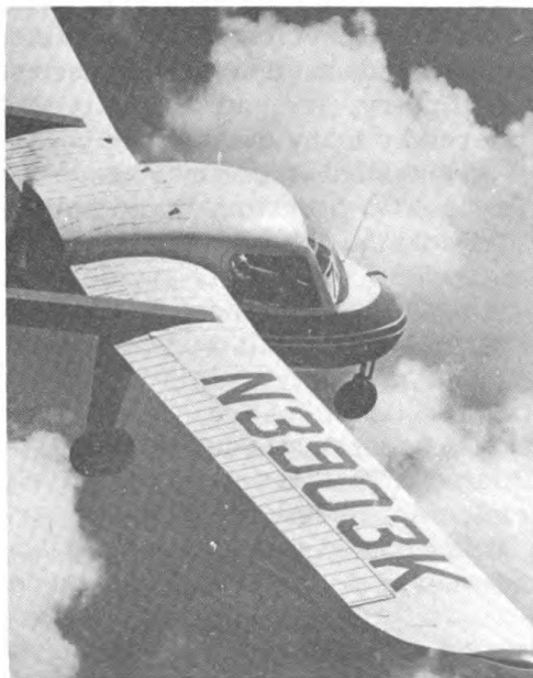
Figure 3 - Tufts of woolen yarn affixed to the skin of a Pusher Airplane AG-14 demonstrate air flow over wing and fuselage. A F9F-4 has proved the value of boundary layer control.
