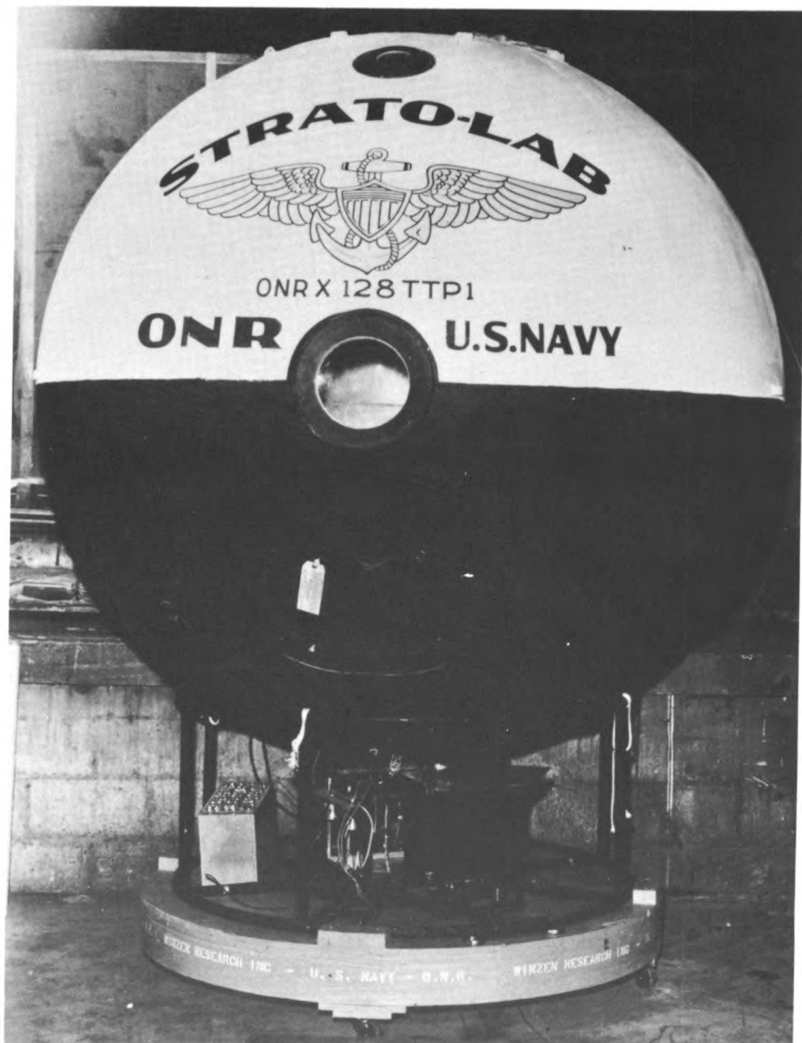
The STRATO-LAB system has special instrumentation for gathering scientific information while aloft and for radio communications with stations on the ground.
