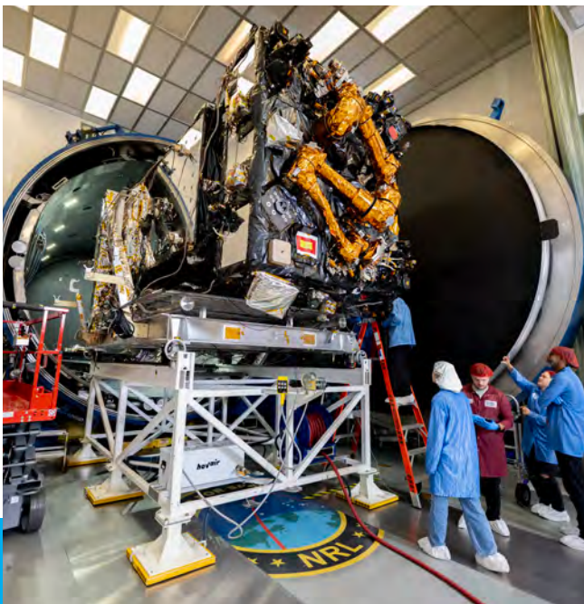
The Robotic Servicing of Geosynchronous Satellites (RSGS) payload integrated with the Northrop Grumman Mission Robotics Vehicle (MRV) spacecraft bus sits outside the cryogenic thermal vacuum chamber after completing testing at the U.S. Naval Research Laboratory’s (NRL) Naval Center for Space Technology (NCST) in Washington, D.C. NRL NCST, with funding support from the Defense Advanced Research Projects Agency (DARPA), conducted the final space-readiness testing on RSGS, a robotic payload designed to extend and upgrade satellites already in orbit. (U.S. Navy photo by Jonathan Steffen-Arnold)
