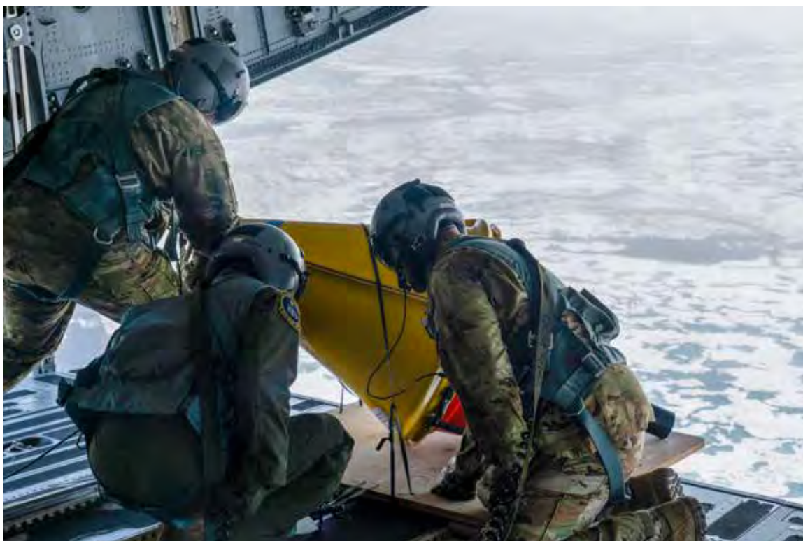
Alaska Air National Guard loadmasters assigned to the 144th Airlift Squadron prepare to deploy an Air-Deployable Expendable Ice Buoy (AXIB) in the Arctic Ocean. (U.S. Air Force photo by Airman 1st Class Shelimar Rivera Rosado)
