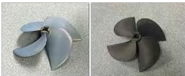
3D Maint. Bn Marines scanned the T-12 propeller (right) and successfully printed / fabricated the same propeller(s) during AW23.2 in Jervis Bay, Australia. (Photos courtesy of ONR GLOBAL)
