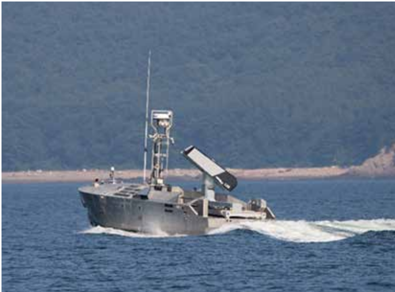
Fast Inshore Attack Craft fitted with 2.75 inch Poniard rockets. (Photos courtesy of South Korea and ONR GLOBAL)
