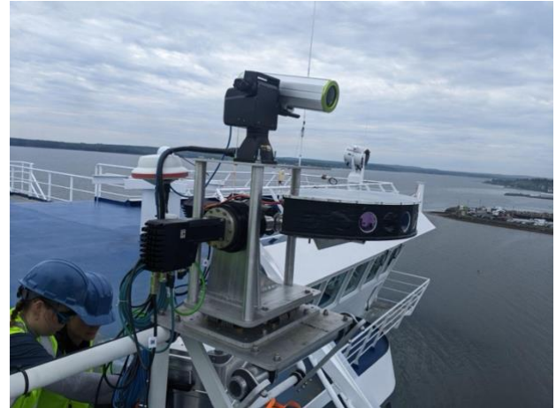
Figure 1) Whale detection system installed on MV Blue Puttees
