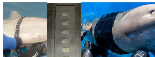
Fig.1. Dolphin electrode-belt designs. (Left) original design with cables and electrode clips. (Mid) modified belt/vest design uses a neoprene layer to cover electrodes (Right) Dolphin wearing new design
