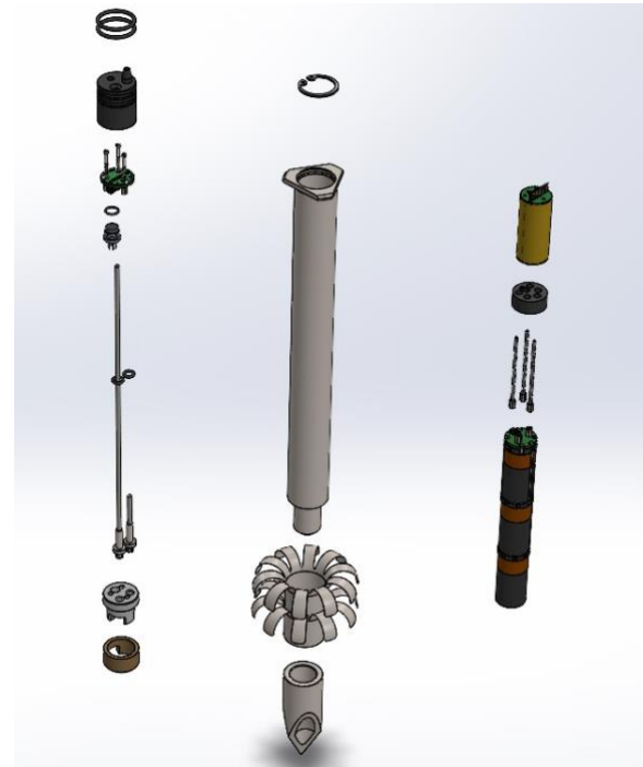
Figure 1: Visualization of the robust tag housing (middle) with re-designed endcap assembly (left) and internal electronic components (right)
