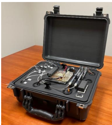
Figure 1: 16"X13"X7" portable instrument with attached eDNA analysis cartridge.
