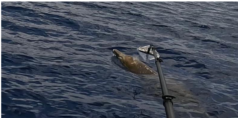
Figure 1. Noninvasively collecting exhaled respiratory vapor from a Blainville's beaked whale, using a polystyrene dish fastened to the end of a long pole and positioned above the exhaling blowholes; collected under The Bahamas Department of Environmental and Planning research permit BS-2023-177568.
