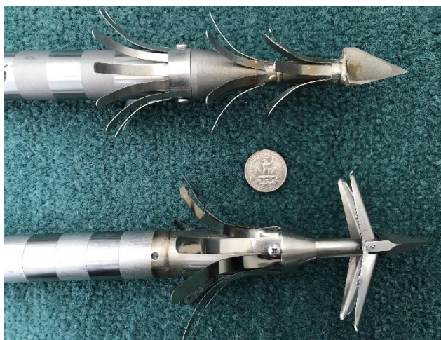
Fig. 1 – Type I tags with three bladed tip and three sets of retention elements (top) and two bladed tip with two sets of retention elements (bottom). Note that retention elements are shown in deployed position in both designs.
