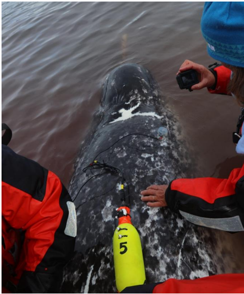
Fig. 1. ECG-ACC-Depth monitor deployed on a narwhal in Scoresby Sound, Greenland. The tag is placed on the skin by suction cups and falls off after 1- 4 days.
