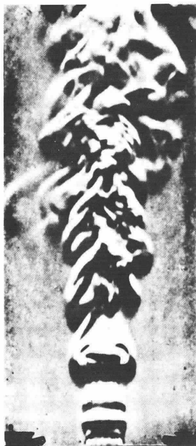
Fig. 7 - The flow of jet-tones. Flow separation occurs within the orifice and the periodic shedding of the vortices with the associated fluctuation in flow results in the characteristic toroidal vortex formations. (From a photograph by W. H. Darlington (50).)
