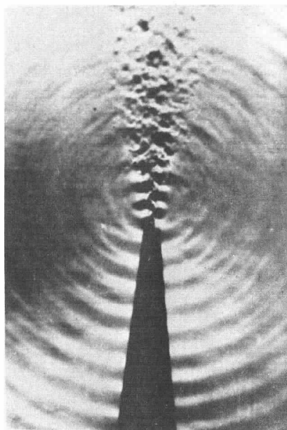
Fig. 10 - Choked-jet noise. The flow is very similar to that for high-speed edge tones; but here the interaction of the eddy formations with the regularly spaced standing shockwaves produces the sound. The jet pressure is considerably higher than the edge-tone case of Fig. 5. (This photograph is by M. G. Davies (62).)
