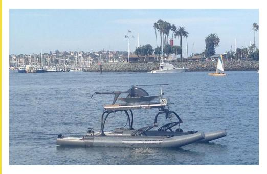
The MCM C2 combines air, surface and sub-surface unmanned assets for the first time to speed the operational pace and reduce the detect-to-engage timeline in naval mine warfare. It also enables military personnel to operate further away from high risk areas.
