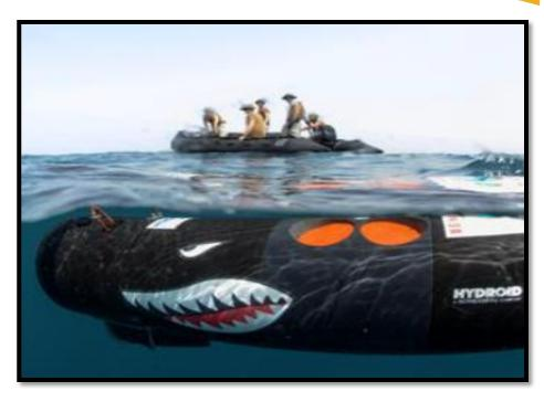
NOMWC UUV Platoons have significant expertise operating in ports, harbors, confined waterways, and in open ocean operations. Platoons operate a system (3) of Mk 18 Mod1 Swordfish UUVs from Naw RHIB boats.
