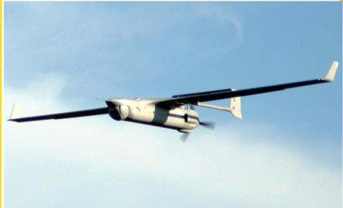
The NRQ-21 system provides persistent maritime and land-based tactical reconnaissance, surveillance, and target acquisition (RSTA) data collection and dissemination capabilities. The air vehicle's open-architecture configuration can integrate new payloads quickly and can carry sensor payloads as heavy as 25 pounds. Payloads could include day/night full-motion video cameras, infrared markers, laser range finders, communications relay packages and automatic identification system receivers.
