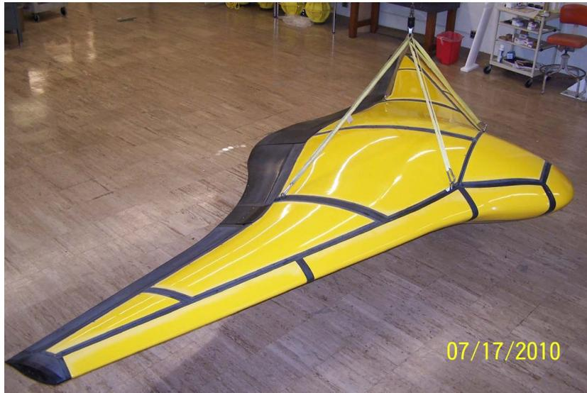
**Figure 1. Photograph of ZRay, suspended from its three lift points in the laboratory without its 3-ft antenna mast or wing tips installed.**
