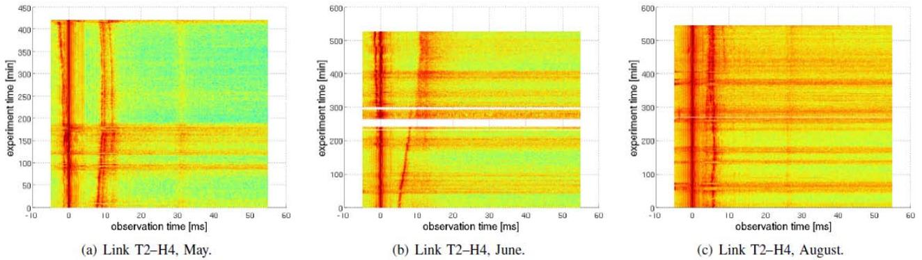
**Fig. 3: Pseudocolor plot of measured channel impulse response amplitudes for the link between T3 and H4.**
