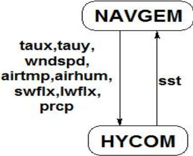
*Figure 3 A system of NAVGEM coupled with HYCOM*
