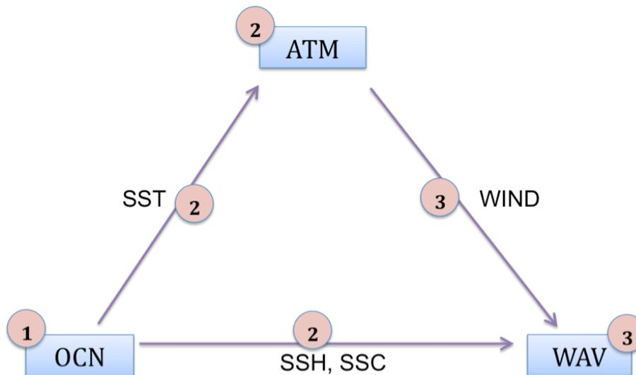
**Figure 2** Graphic depicting how the initial inter-model data dependencies are resolved. Arrows indicate a data-dependency of a model that must be satisfied before the model initial state can be computed. The circled numbers indicate the order in which model initialization and connectors are executed.
