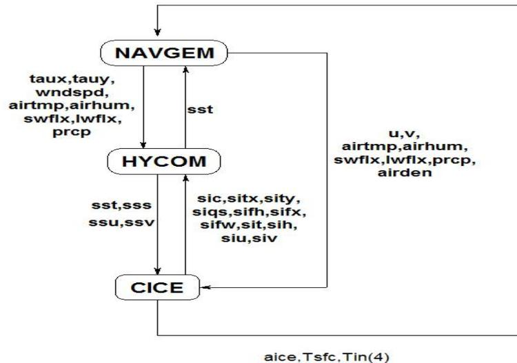
**Figure 6 A system of NAVGEM coupled with HYCOM and CICE**
